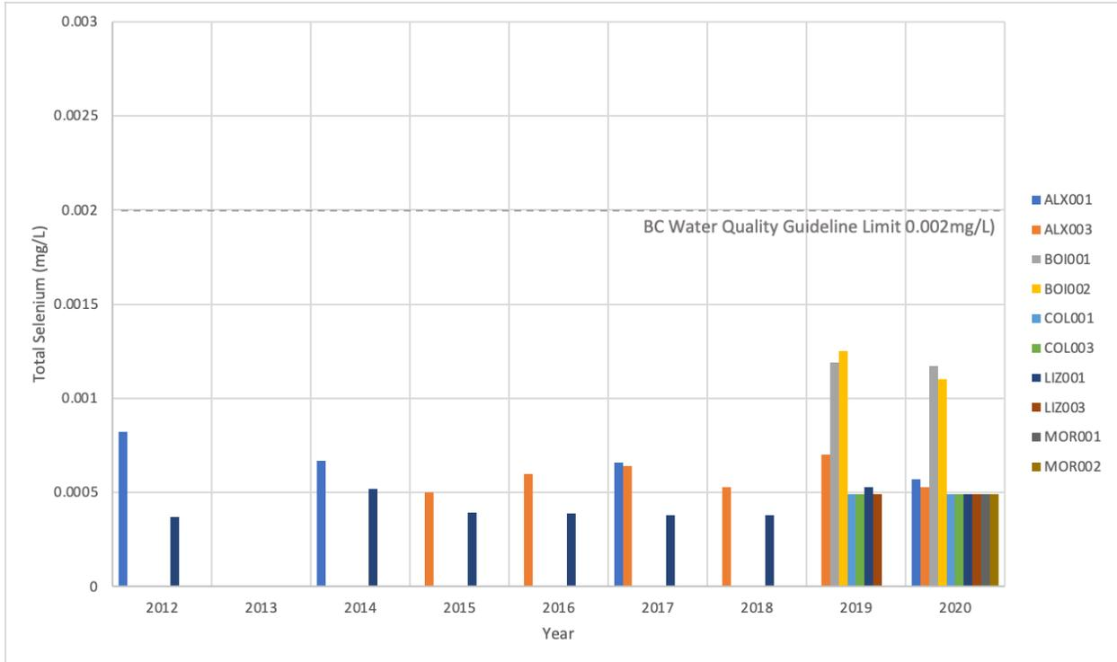
Figure 40. Total seleniun concentrations at CBWM sites from 2012 to 2020. All concentrations are well below the BC water quality guideline of 0.002 mg/L (2µg/L).
