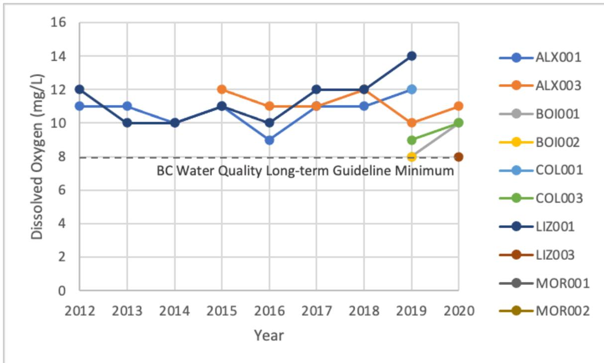
Figure 37. The amount of dissolved oxygen at CBWM sites in mg/L from 2012-2020. Site values do not fall below the BC water Quality Long-term Guideline minimum for Freshwater Aquatic Life (8mg/L).
