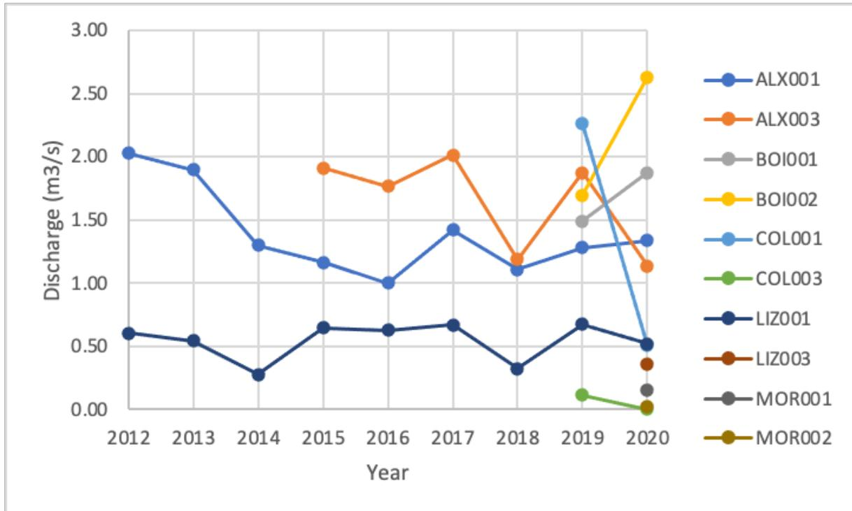
Figure 38. Discharge measurements calculated for CBWM sites from 2012- 2020.
